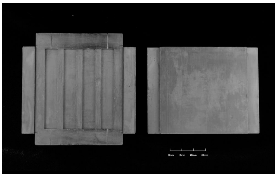
Figure 2 Stainless steel mold for making specimens.
